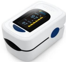
A pulse oximeter is a medical device that measures how efficiently oxygen being breathed into our lungs is reaching our blood stream.
